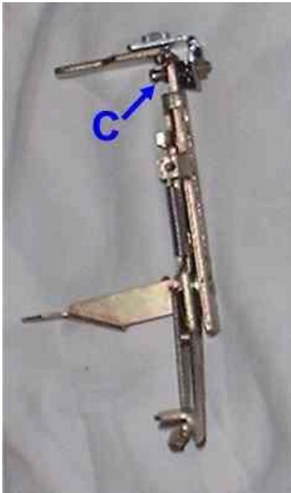
The third adjustment is uncommon. Clearance of 0.6mm between the ribber needles when pushed up and the sinker posts of the main bed is recommended. Try sliding a punchcard or sheet of quality writing paper down between them to judge if they are too close (it won't fit), and a c.d. to see if they are too far apart. If the carriages do not seem to want to connect, or there is obviously pressure on the connector, then this might cure it.
