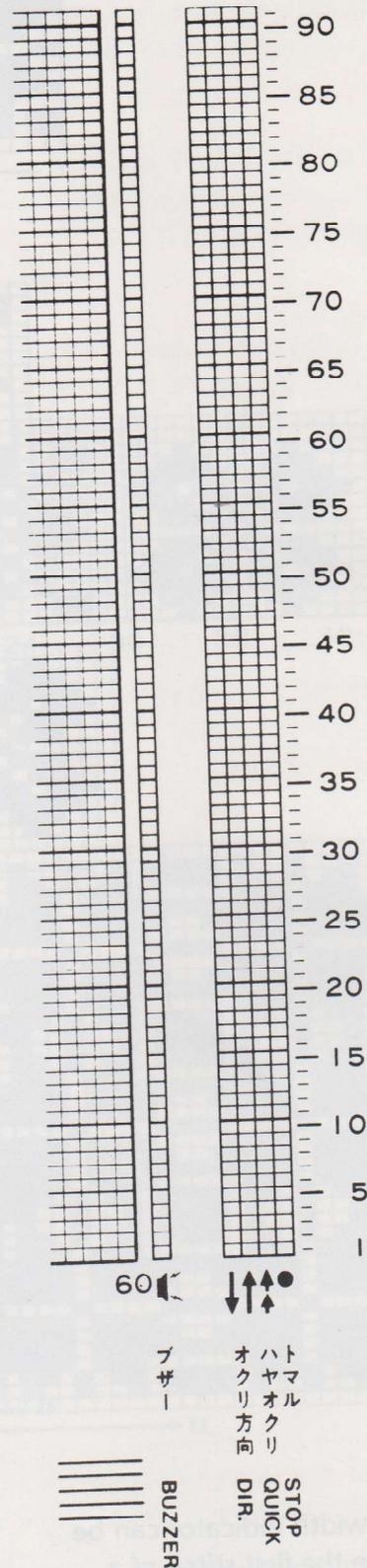
2: The scanners read the buzzer and direction columns for each row of the design.
