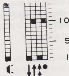
**3C: The card is marked to read from top to bottom with a quick return to the first (top) row.**
